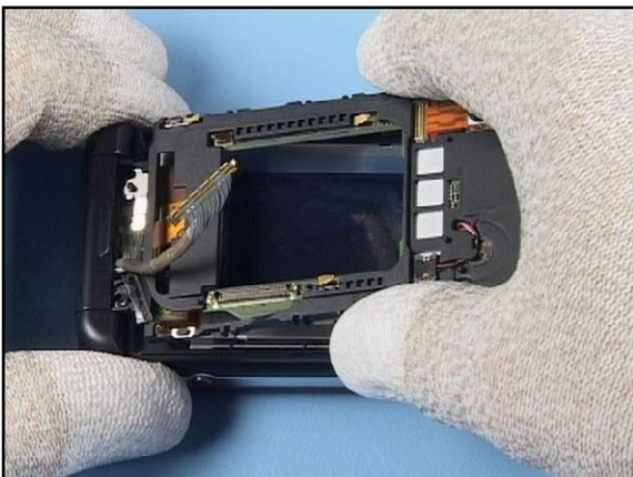
17. ...and remove it from the A-COVER ASSY.
