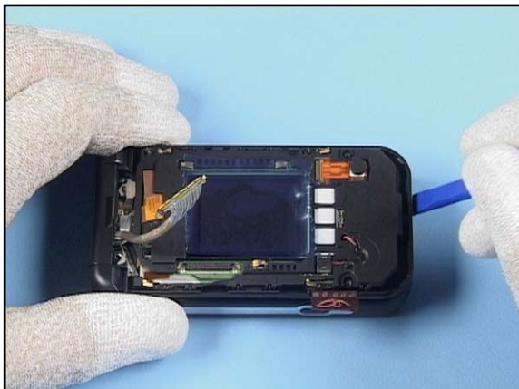
16. Unlock the UPPER C-COVER ASSY using the SS-93...
