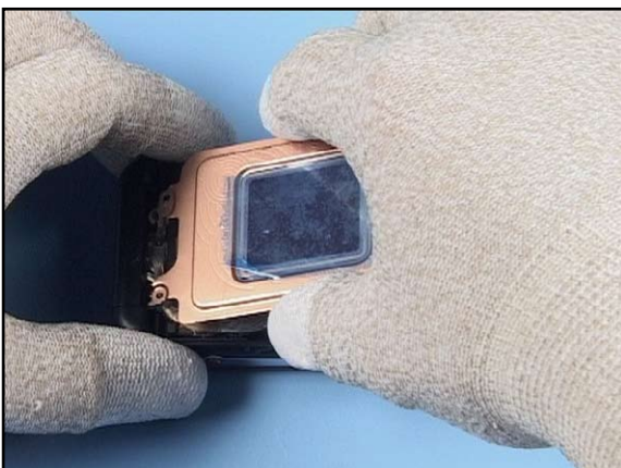
11. Remove the SECOND DISPLAY FRAME ASSY.
