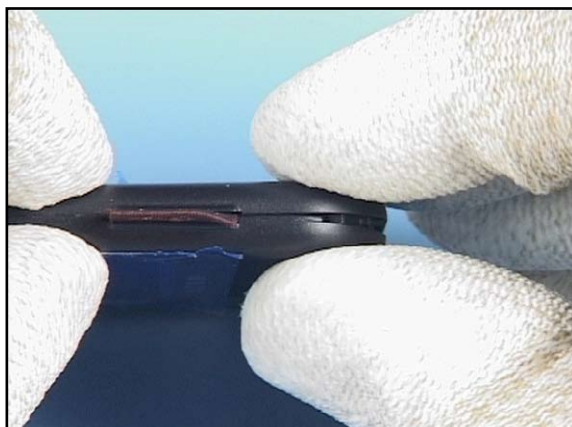
24. ...and secure it by squeezing the covers.
