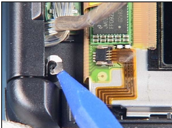
10. Lift the metal tab as shown...
