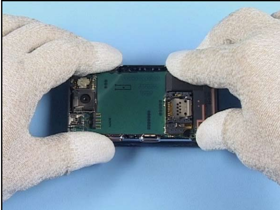
13. Fit the ANTENNA ASSY.
