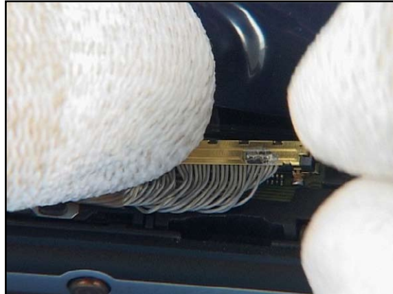
14. After covering the display, gently close the COAX CONNECTOR.
