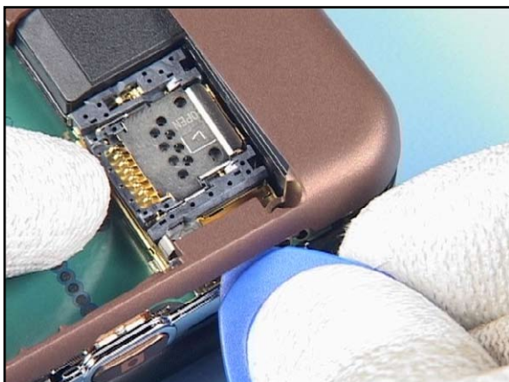
12. ...unlock the remaining snaps and remove the LOWER B-COVER.
