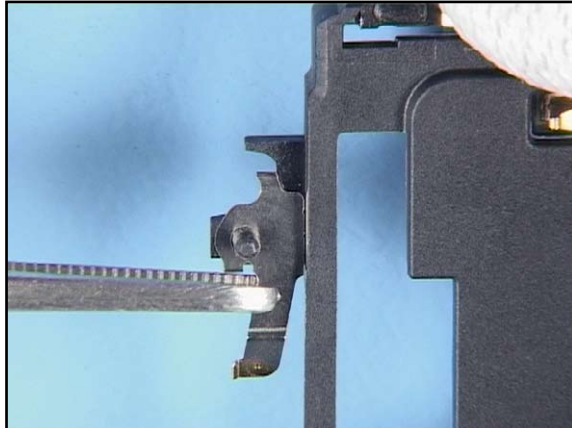
8. Fit the COAX PWB GROUNDING SPRING to the UPPER C-COVER.
