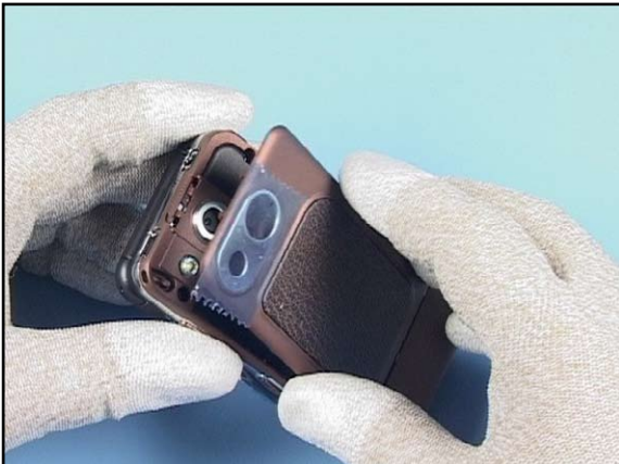
21. Fit the BATTERY COVER.
