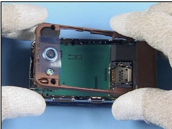
15. Align the LOWER B-COVER with the LOWER A-COVER...
