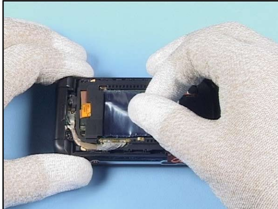
14. Cover the display surface with the protective film.
