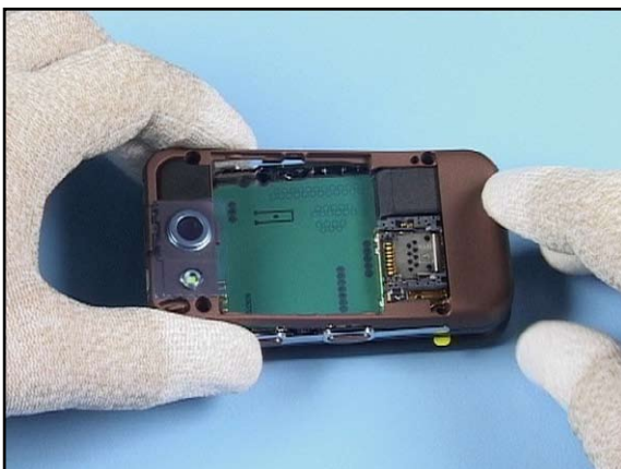
11. Lift a bit the LOWER B-COVER, ...
