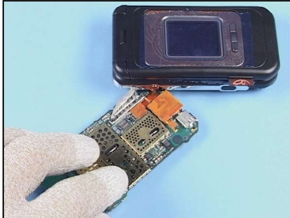
20. ...and than gently place the PWB on the table.
