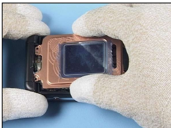
18. Align the SECOND DISPLAY FRAME ASSY with the UPPER C-COVER.
