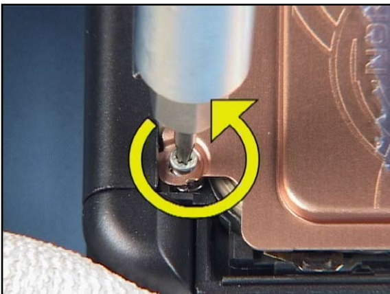
21. To avoid damaging the threads first turn the screws slightly left to engage the threads and then tighten them lightly.
