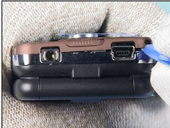
8. Start to release the LOWER B-COVER by opening the snaps on the shown side.
