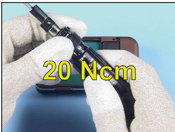
18. Set the torque driver to the torque of 20 Newton centimeter.
