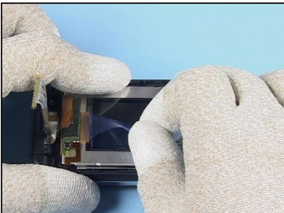
9. Now, remove the protection film.
