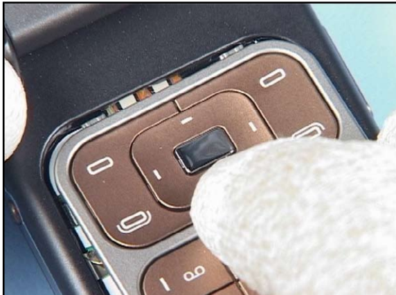
22. Place the KEYMAT onto the LOWER A-COVER...
