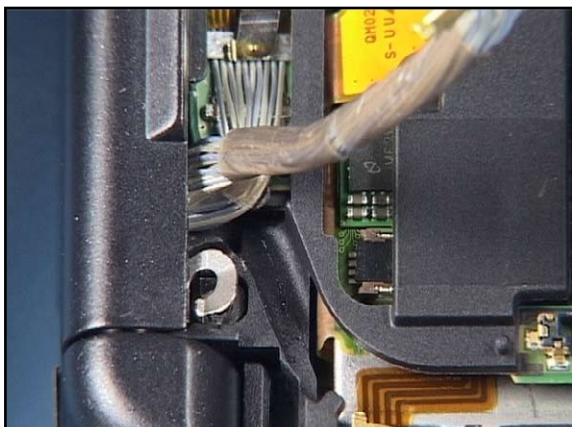
12. Pay attention to the right position of the metal tab. It must be placed over the screw hole of the UPPER C-COVER.
