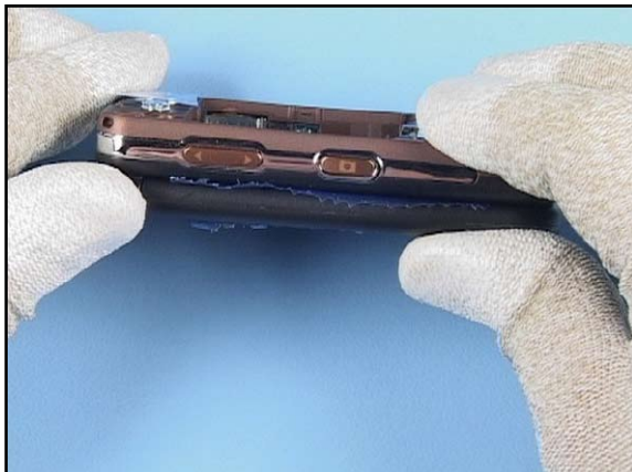
16. ... and gently press the covers together.
