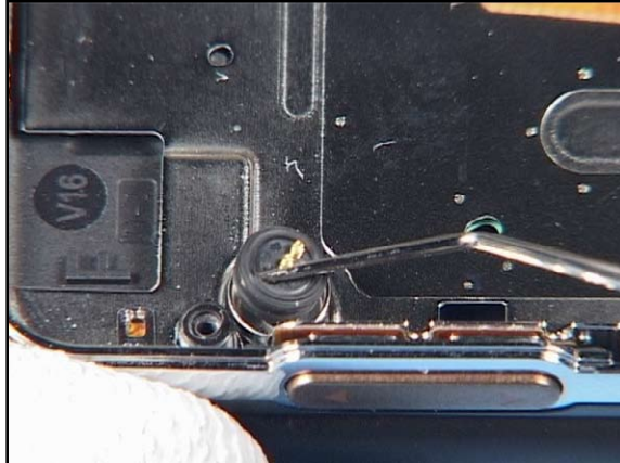
26. Remove the MICROPHONE.
