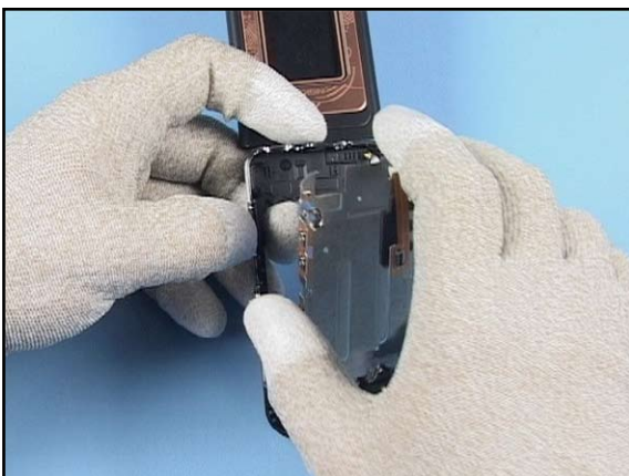
29. and remove the LOWER C-COVER ASSEMBLY.
