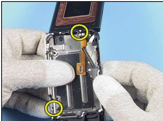
28. Bend a bit the LOWER A-COVER to release the metal clips of the LOWER C-COVER.
