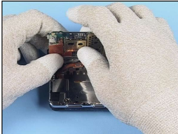
8. Lift up the PWB and hold it as shown...
